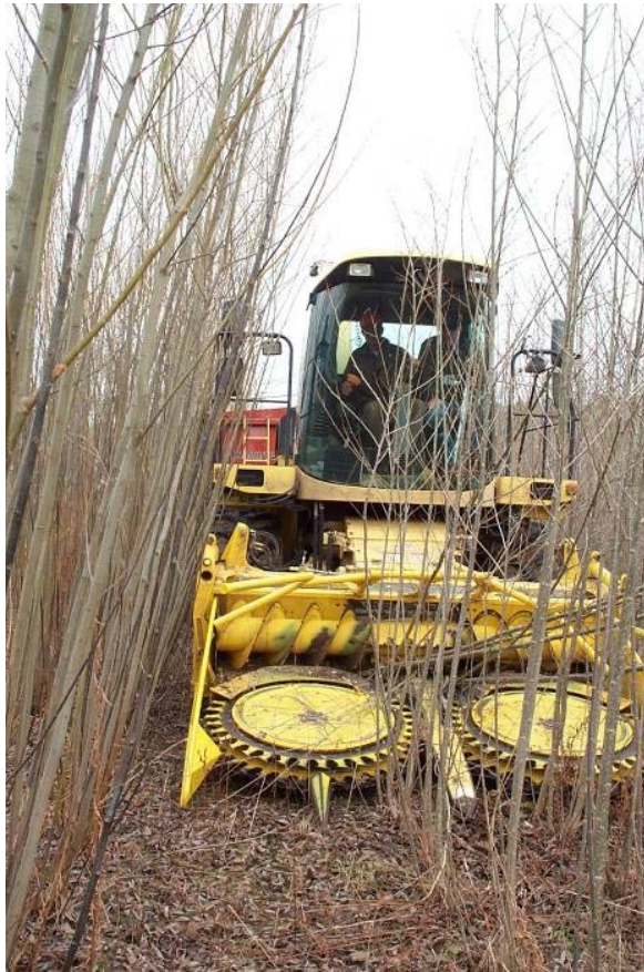
Figure 2: New Holland FX45 forage harvester with a modified row independent (Kemper) corn head harvesting 3-year-old willow biomass crops during field trials in December 2004 and January 2005 at the SUNY-ESF Genetic Research Field Station in Tully, NY.
