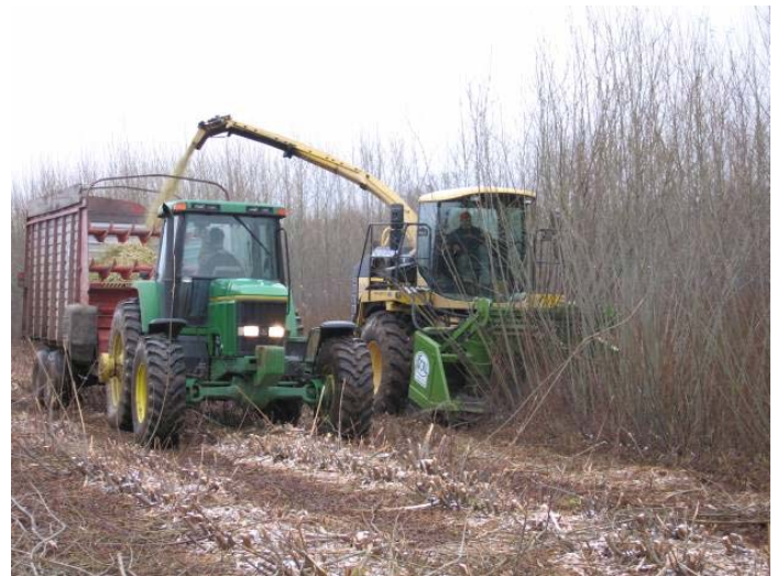
Figure 3: Harvesting willow biomass crops with a New Holland FX45 forage harvester and a specially designed Coppice Resources Ltd. (CRL) willow cutting head in NY during fall 2006. The chips are being blown into a large tandem forage wagon and tractor which will haul the chips to the field edge to be loaded into a chip trailer.
