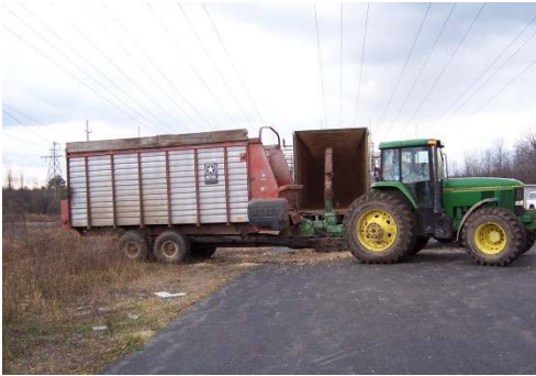
Figure 4: The large tandem forage wagon in position to unload harvested willow chips into a forage blower which in turn will blow the chips into the chip trailer for hauling over the road to the end user.
